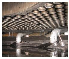
Sugar Research Institute's Jigger Tube System improves massecuite circulation, energy efficiency and pan performance.
